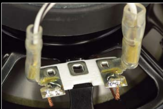
Installing a universal speaker requires cutting the wire so it fits the speaker correctly.
