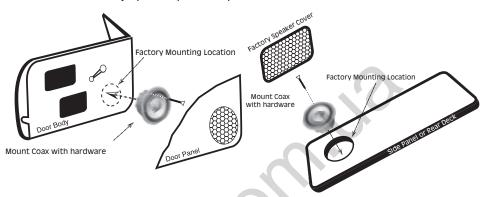
If custom mounting locations are desired for your drivers, check for interference from other mechanical systems in the vehicle. Watch for window mechanisms, hinges, trunk springs, wire harnesses, and anything that would be affected by the installation of these drivers. If metal must be cut to mount the speakers, try to avoid structural metal and braces. Once a location is chosen, cut the appropriate size hole for the drivers.
