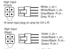
Hi level input plug on amp for CH  $\ensuremath{\text{L/R}}.$
