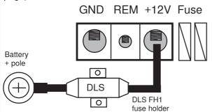
A cable up to AWG 4 fits directly in the amplifier + 12 V terminal, tighten with the hex screw.
