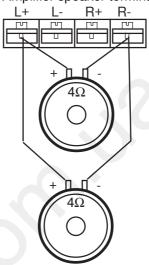
Single voice coil subwoofer connected in bridge mode. Impedance = 2 ohm Amplifier load = 1 ohm (only for DLS A-series amplifiers)
