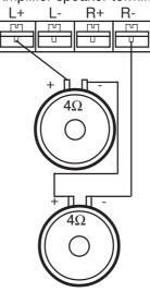
Connection of two subwoofers with 4 ohm voice coils in series Impedance = 8 ohm Amplifier load= 4 ohm
