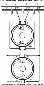
Connection of two subwoofers with 4 ohm dual voice coils Impedance = 1 ohm
