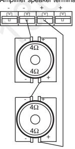
Connection of two subwoofers with 4 ohm dual voice coils in parallel and then in series to the amplifier with a resulting impedance of 4 ohms.
