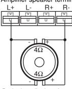
On DLS mono amplifiers, with dual speaker connectors, both the + and - terminals are internally connected in parrallel.
