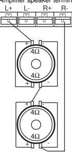
Connection of two subwoofers with 4 ohm dual voice coils in parallel and then in series to the amplifier gives a resulting impedance of 4 ohm. Amplifier load = 2 ohm
