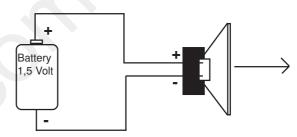
**NOTE!** Tweeters can not be tested this way, double check the connections instead.
