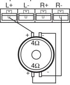
Connection of a 4 ohm dual voice coil subwoofer with the voice coils in series. Impedance = 8 ohm Amplifier load= 4 ohm
