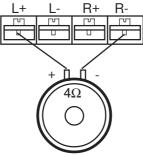
Single voice coil subwoofer connected in bridge mode. Impedance = 4 ohm Amplifier load = 2 ohm
