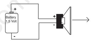
**NOTE!** Tweeters can not be tested this way, double check the connections instead.
