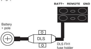
A cable up to AWG 4 fits directly in the amplifier + 12 V terminal, tighten with the hex screw. RM20 handles AWG5 (16 mm<sup>2</sup>.)
