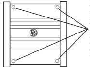
Remove these screws using a 3 mm hex. key for removal of side flange. Remount after fastening the amplifier and connection of the speaker and power cables.
