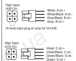
Hi level input plug on amp for CH C/D.
