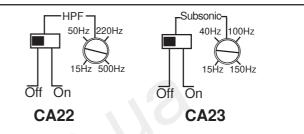
The **HPF** (high pass filter) blocks very low frequencies from reaching the speakers. It is mostly used at say 60 Hz to protect small speakers (like 6 inch and smaller) from deep bass. It can also be used as subsonic filter to take away the very deepest frequencies from a bass box. The typical setting is then around 25-40 Hz. In CA23 the high pass filter is designed as a subsonic filter variable from 15 Hz to 150 Hz.
