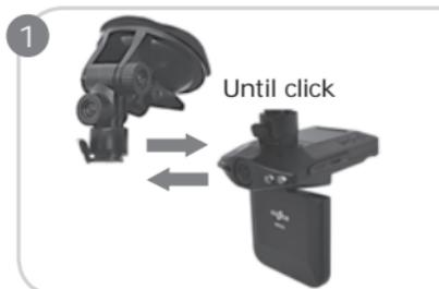
Connect the frame of the device with the mount.
