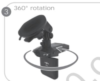
You can rotate the recorder in any direction around its axis.
