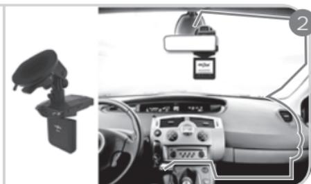
Install the MVR and fix the power supply cable as shown in the drawing.
