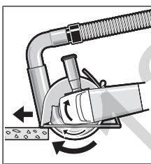
Switch on the power tool and position it with the front part of the guide block on the workpiece. Move the power tool with a moderate feed motion that is suited to the material being machined.
