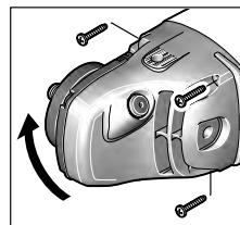
The machine head can be rotated in 90° increments. This enables the on/off switch to be brought into a more convenient position for particular working situations, such as cutting operations using the extraction guard for cutting with a guide block (21) or for left-handed persons.
