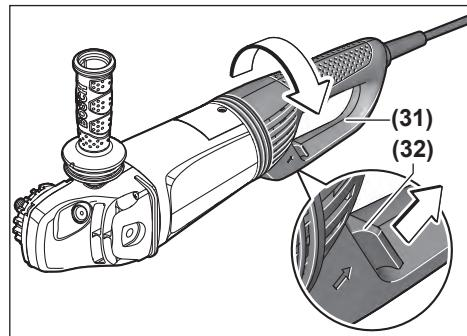
The main handle (31) can be rotated 90° to the left or right relative to the motor housing. This enables the on/off switch to be brought into a more convenient position for particular working situations, such as cutting operations using the extraction guard for cutting with a guide block (21) or for left-handed persons.
