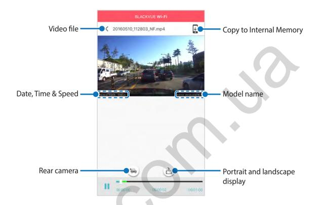
The vehicle's speed is displayed in the lower-left corner of the video.
