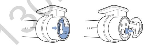
Peel off the protective film from the double-sided tape and attach the front camera to the windshield behind the rear-view mirror.
