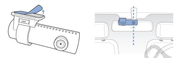
Adjust the angle of the lens by rotating the body of the front camera. We recommend pointing the lens slightly downwards (≈10° below horizontal), so as to record video with a 6:4 road to background ratio.
