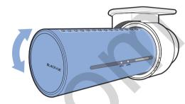
Peel off the protective film from the double-sided tape and attach the rear camera to the rear windshield. Adjust the angle of the lens by rotating the body of the rear camera.
