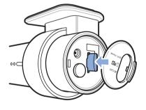
Peel off the protective film from the double-sided tape and attach the dashcam to the windshield behind the rear-view mirror.
