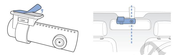
Adjust the angle of the lens by rotating the body of the dashcam. We recommend pointing the lens slightly downwards ( $\approx$ 10° below horizontal), so as to record video with a 6:4 road to background ratio.
