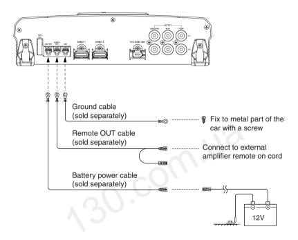
When connecting the Battery power cable direct to the battery terminal, a fuse at the battery should be used to protect your equipment. Please consult with your Alpine dealer for the proper fuse value.
