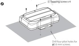
Drill the pilot holes for  $\phi$ 3.6 mm screws on the sheet metal section of the vehicle , and attach the speaker unit to the vehicle using the tapping screws (5).
