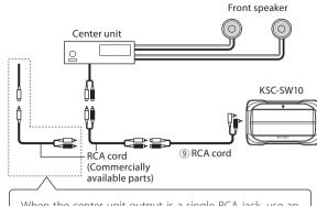
When the center unit output is a single RCA jack, use an RCA cord that converts the output into the two RCA jacks as shown above.
