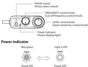
The illumination on the subwoofer turns on and off in an interlocked operation with the PWR indicator on the remote control unit.
