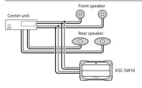
Connect the subwoofer to the front or rear output cords of the center unit.
